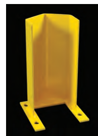
7" x 7" x 1/4" Base Plate with the industry's widest throat increasing space between rack post and protector allowing protector to absorb impact without hitting the post
