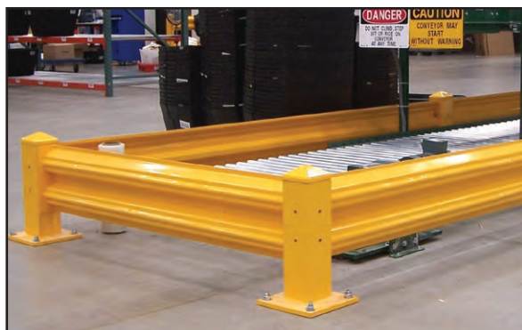
Steel post cap snaps on providing a durable finished installation
